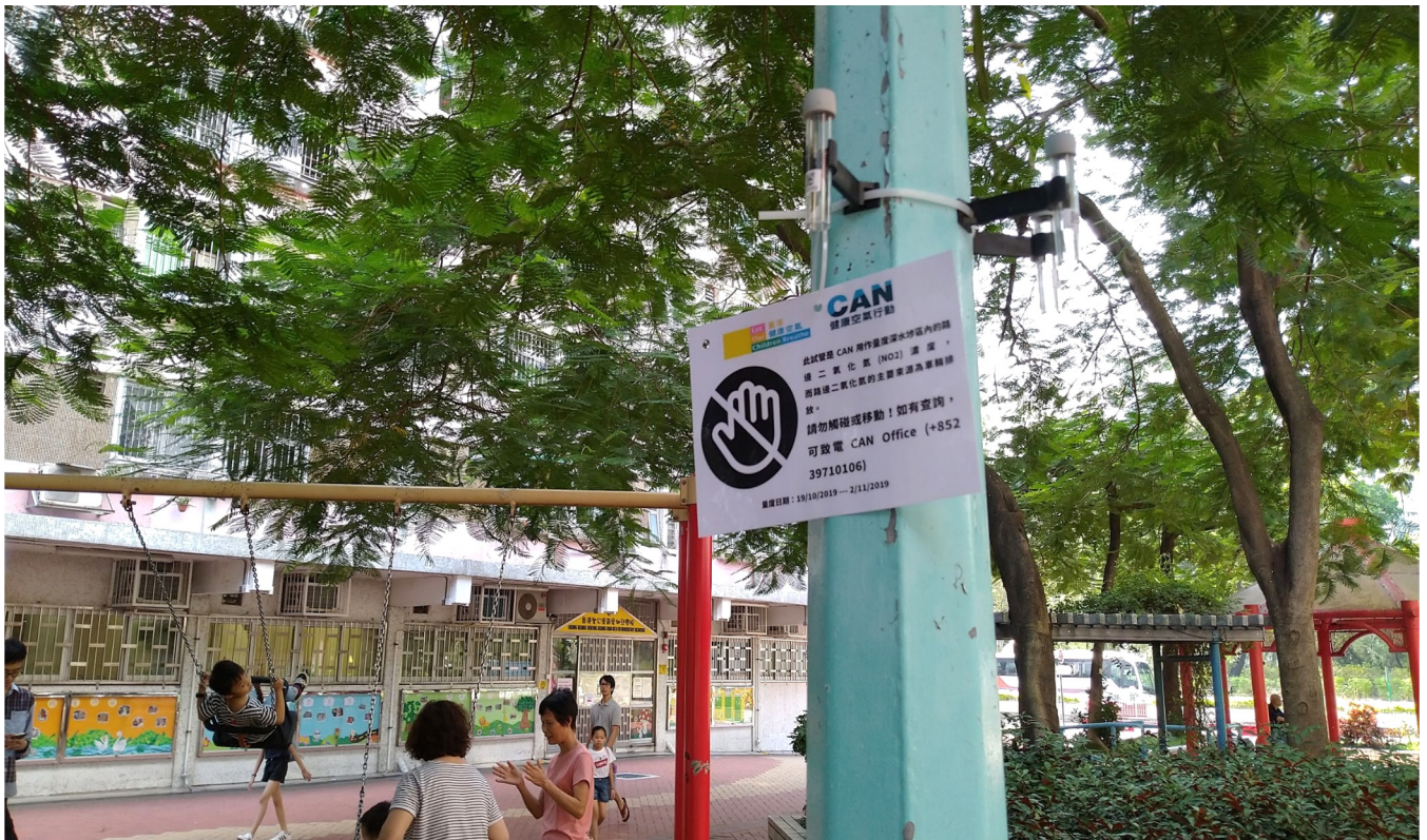
Photo 1: NO 2 diffusion tubes installed at Sham Shui Po Park Stage II
