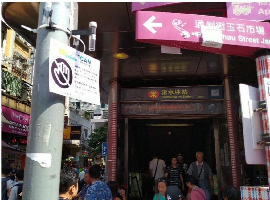
Photo 2: NO2 diffusion tubes installed at Sham Shui Po MTR Station C2 Exit
